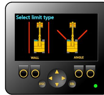
The slew limit type selection is available when the slew limit is first switch ON. The option will remain until the limit is switch OFF again.
