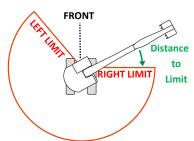
**Note:** If the machine has an offset boom with proximity switch detection, both slew left and right will be prevented if the boom is not central.
