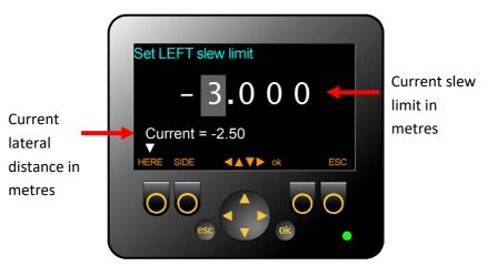
When setting slew walls when the machine is slewed over the rear of the machine, the left limit will actually be on the operators right hand side. This is because the walls are with respect to the undercarriage.
