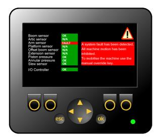
The system continuously monitors the health of the sensors and the IO Controller inputs and outputs. If a problem is detected, the screen shown above will appear. If the system has motion control valves fitted, the system will failsafe and close all the valves. The failed sensor(s) will be shown in red.
