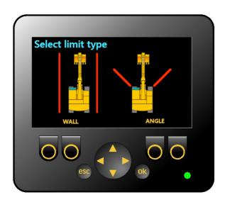
With the exception of XW3, the slew limit type page will appear when the slew limiter is first enabled. Press WALL for left and right slew walls, or ANGLE for left and right angular limits.
