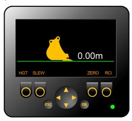
Once referenced, the displayed depth value will represent the true elevation of the excavation base as long as the bucket is in the flat orientation.
