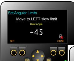
**1.** Slew to the required left slew limit and press **SET**.
