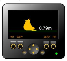
On initial entry to the dig page the depth displayed will be the current lifting point height (usually the bucket pin). Place the bucket flat at the reference elevation and press **ZERO**.
