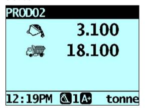
3) Roll the bucket partially forward, tipping product into the truck. The Indicator will give a live weight as it is tipped into the truck.
