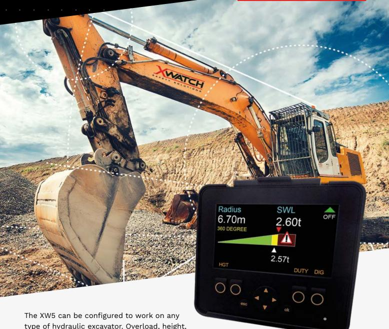
type of hydraulic excavator. Overload, height, and slew limitation are controlled using proportional soft-stop hydraulic valves providing accurate and repeatable performance without detriment to the machine. A basic dig depth monitor is available when the RCI is not required. If hazards arise, XW5 will automatically flip to the relevant display page. Tracked machines have automatic sectored lifting duties for over the front/rear operation and over the
