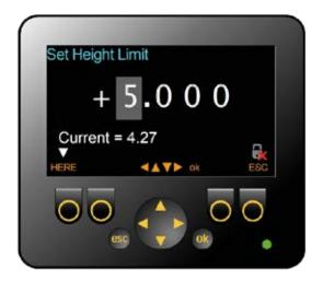
A height limit can be either manually keyed in or set automatically by positioning the machine equipment and pressing HERE.
