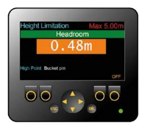
All motions are individually controlled with ramped slow down on approach and soft-stop. There is no machine 'bounce', overshoot, or undershoot. An optional chassis sensor can be installed to correct for terrain slope.
