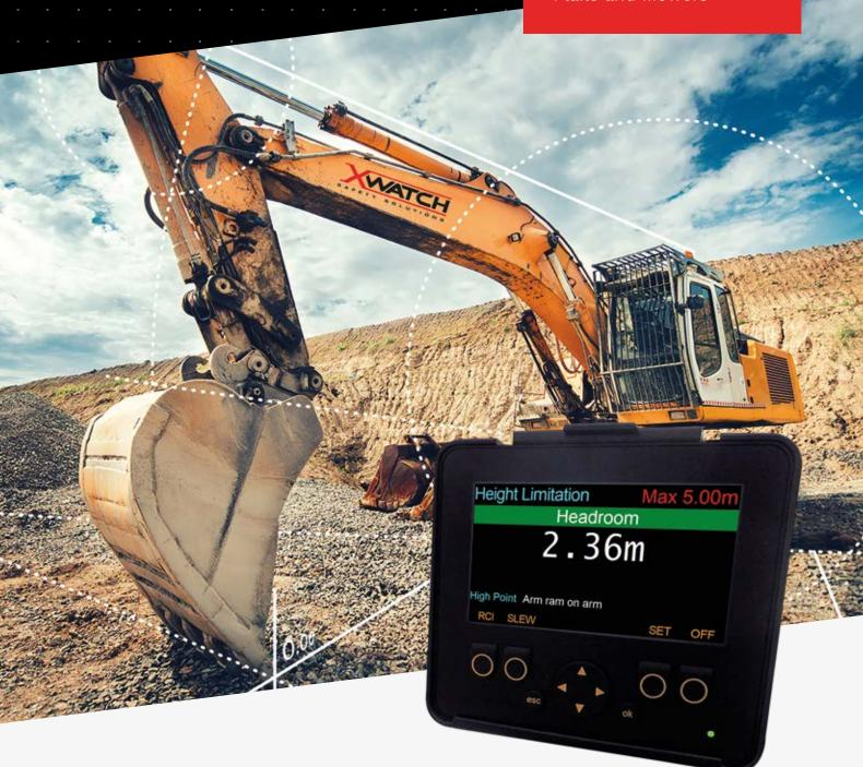
The XW1 can be configured to work on a variety of articulated hydraulic plant. Height limitation is controlled using proportional soft-stop hydraulic valves providing accurate and repeatable performance without detriment to the machine. Operation is fail safe and fully automatic with function selection never more that two key presses away.
