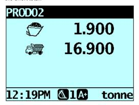
3. Roll the bucket partially forward, dumping the product. The Indicator will display the weight in the bucket and the potential weight of the truck.
