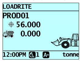
5. Raise a bucketload of product smoothly past the Trigger Point using constant engine revs. The message **Weighing** will display.
