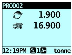
Roll the bucket partially forward, dumping the product. The Indicator will display the weight in the bucket and the potential weight of the truck.
