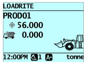
5) Raise a bucketload of product smoothly past the Trigger Point using constant engine revs. The message **Weighing** will display.
