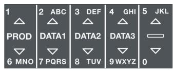
Data field values can be selected before starting a new load. The following example assumes that **Data 1** has been configured to hold customer names and shows how to select a customer name to record against the weighing data.
