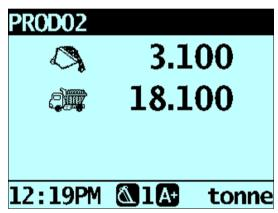
3) Roll the bucket partially forward, tipping product into the truck. The Indicator will give a live weight as it is tipped into the truck.
