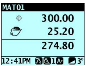
5) As the truck is loaded, the target amount will decrease. The aim is to get as close to 0 (zero) as possible. A positive To load value is under the target; a negative To load value is over the target.
